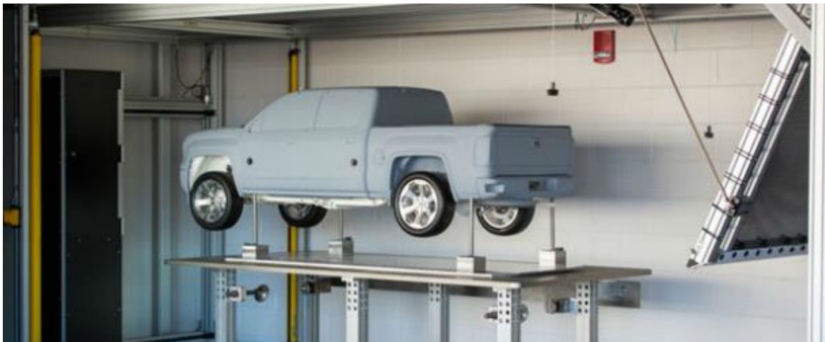
Figure 5. A 3D-Printed 40%-Size Model of a GM Truck Created for Wind Tunnel Testing. Source: Hesel (2015).
